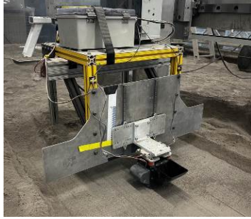
Figure 2. PACT and surface preparation grader blade on the ETS above a prepared, low-density, graded surface.
